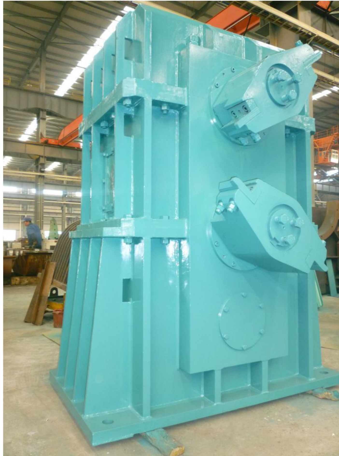
Rolling Mill Gearbox
